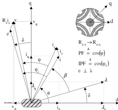
Fig. 3: Vector diagram of SynRM at steady-state, including the total iron losses truster torque
