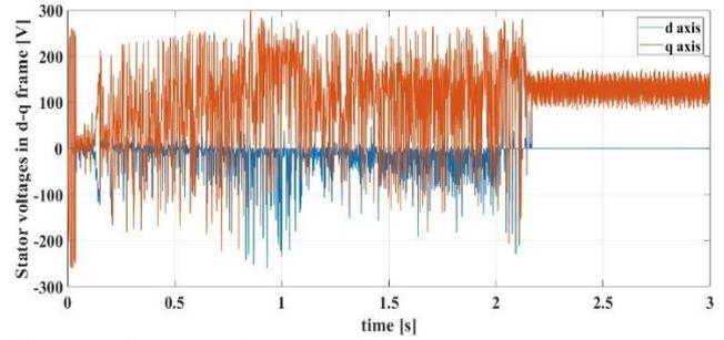
Fig. 11: Stator voltage in  $d,q$  frame
