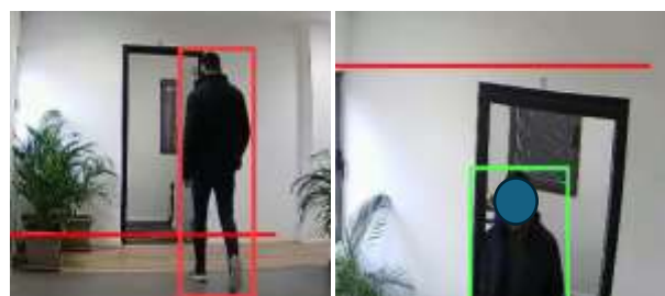
Fig. 10: On the left Line Partition method on straight motion entrance scenario in a location with low altitude. On the right Line Partition method exit scenario in a location with high altitude
