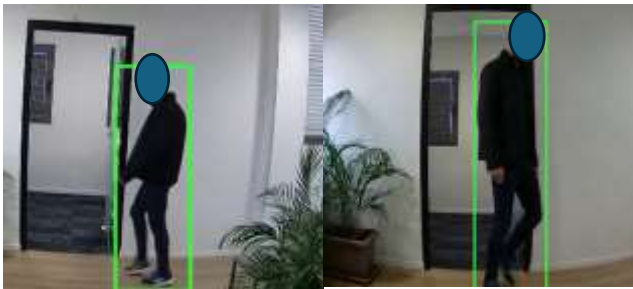
Fig. 11: On the left Bounding Box Diameter method on side motion entrance scenario in a location with middle altitude. On the right Bounding Box Diameter method side motion exit scenario in a location with low altitude
