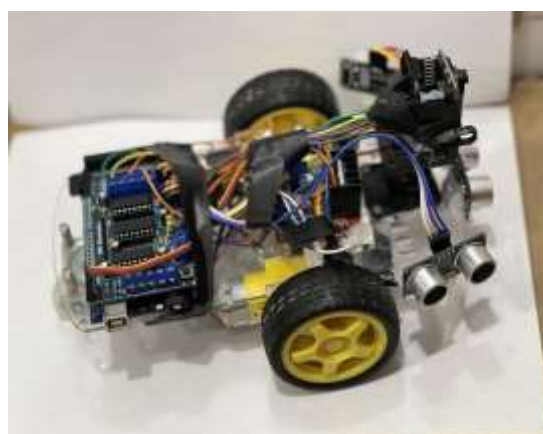
Fig. 20: Image of the physical prototype of a mobile robot.
