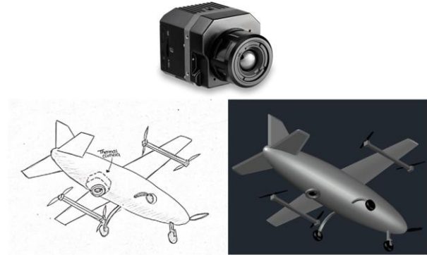
Figure 5: Thermal camera and its location
