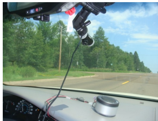
Fig. 10 The LDW system showing the in-vehicle camera and the alarm speaker.
