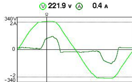
Fig.17 PC and monitor's voltage and current (idle mode).
