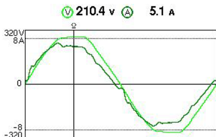
Fig.10 Induction heat plate's voltage and current (load operation, first kettle, 470 ml water).
