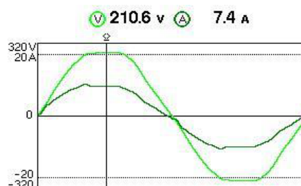
Fig.13 Induction heat plate's voltage and current (load operation, second kettle, 470 ml water).
