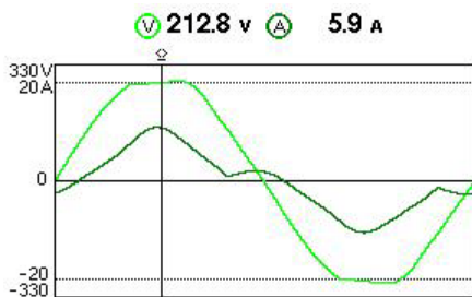
Fig.4 Microwave oven's voltage and current (no-load operation).
