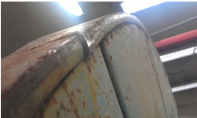
Figure 15: Example of drum sloping flanges
