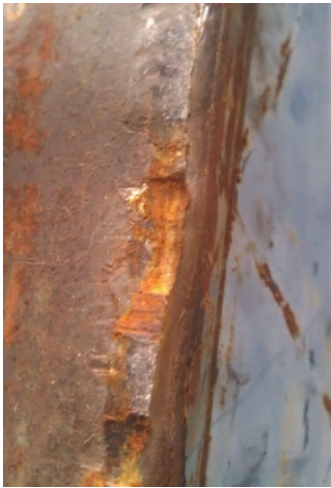
Figure 14: Example of scratch on drum
