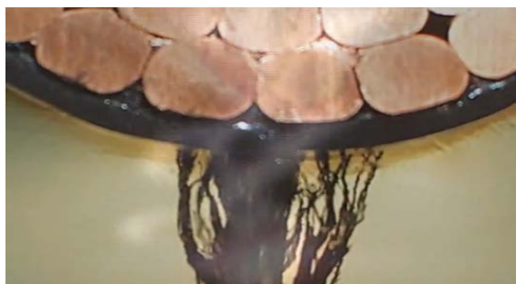
Figure 9: PD phenomenon starting from external semiconductive
