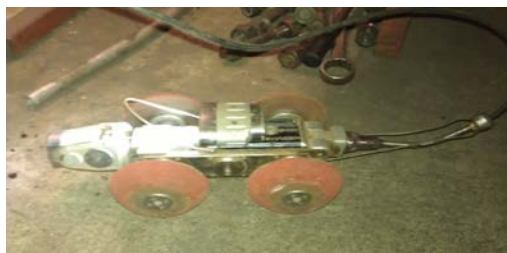
Figure 20: Robot used to check the insulation pipes
