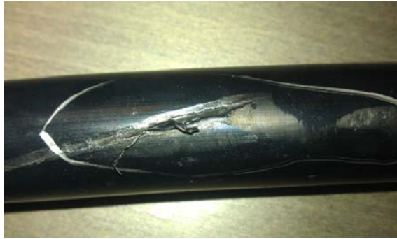
Figure 7: Example of mechanical scratch (1)
