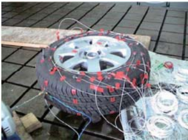
Fig.5 Tire Modal Test
