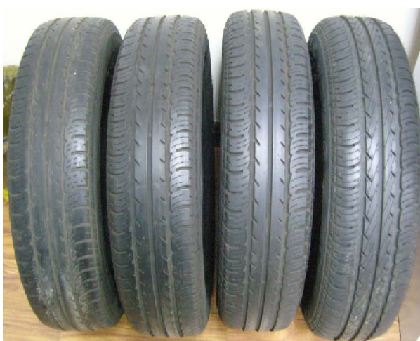
Fig.3 Tire Uniform Wear
