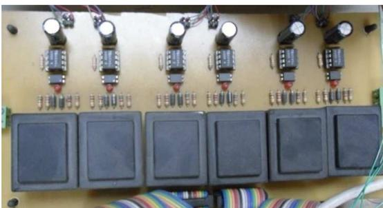
Fig.11 isolation circuit
