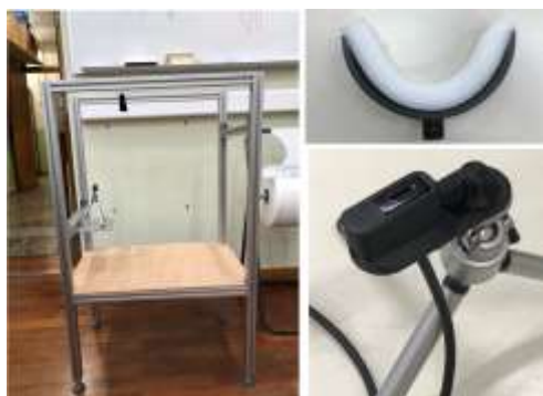
Fig. 2: Thermographic image acquisition: platform (left); footrest (top right) and tripod (bottom right)
