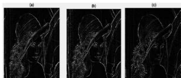
Fig. 10: Results of LoG filter: (a) \alpha = 0.4018 and \beta = 0.0760 , (b) \alpha = 0.2399 and \beta = 0.1233 , (c) \alpha = 0.3685 and \beta = 0.6256
