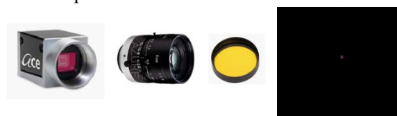
(a) CCD + lens + filter (b) Sample image Fig 9. Image capturing device and sample image taken with IR cut-on long wave pass filter
