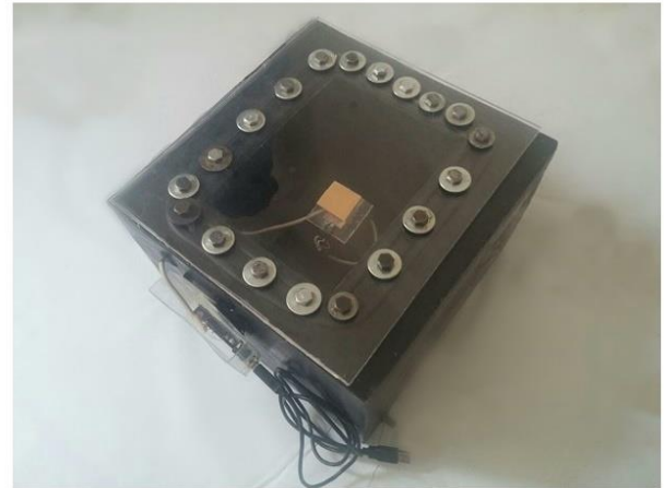
Fig. 2: An overview of the chamber designed for PSP testing
