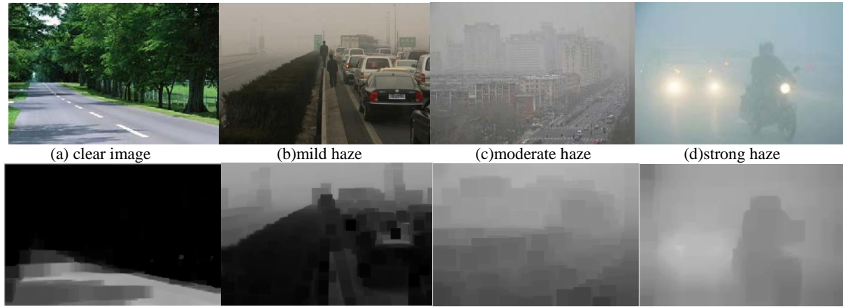
(e)dark color image of figure(a) (f) dark color image of figure(b) (g) dark color image of figure(c) (h) dark color image of figure(d) Figure 1: Dark color images under different haze concentration degree
