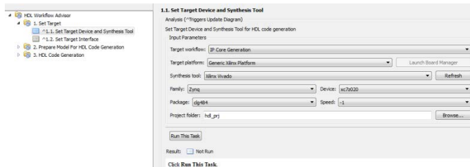
Fig. 10. ZedBoard HDL Workflow Advisor Input Parameters (Set Target)
