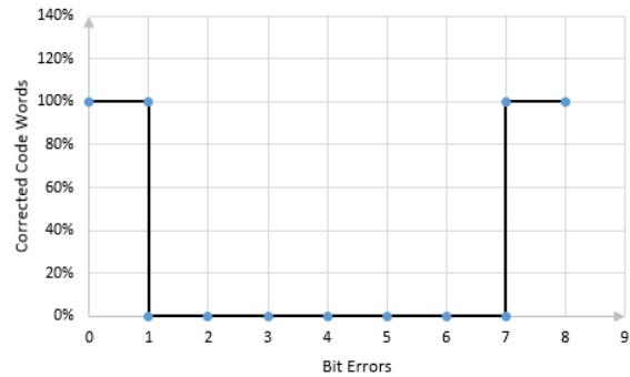
Fig. 1. Error Correcting Capability of 8 Bit Hadamard Code
