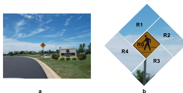
Fig.7. An example of the segmentation process of the four surrounding regions of a warning sign.
