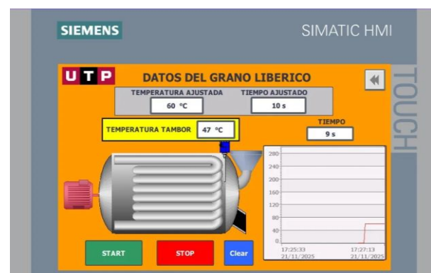
Fig. 20: 20HMI screen in a 60°C control process
