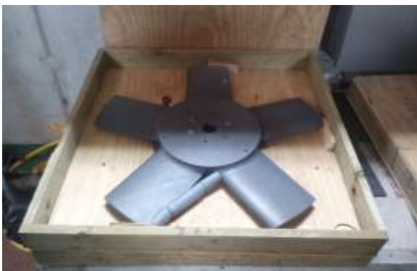
Fig. 3: Unused Wells turbine
