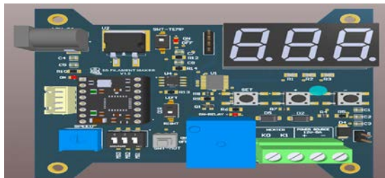
Fig. 5: 3D simulation view of the PCB
