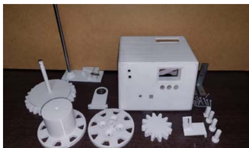
Fig. 8: 3D printed parts and accessories of the foundry machine
