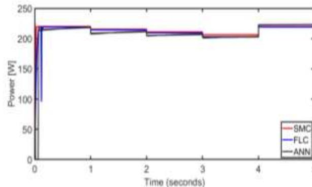
Fig. 6: The power output of the three controllers as the temperature and irradiance levels remain constant.
