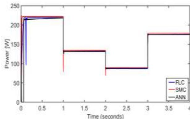
Fig. 5: The power output of the three controllers at a constant 25 C and varying levels of irradiance.
