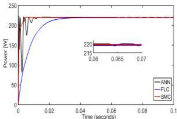
Fig. 4: An analysis of the three controllers in comparison to a constant atmospheric condition
