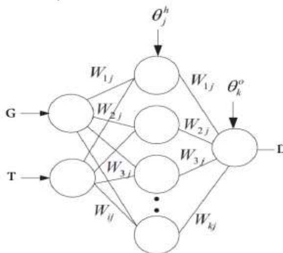
Fig. 3: The construction of the ANN
