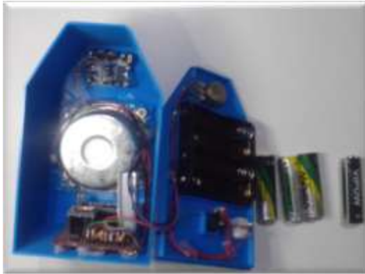
Fig. 10: Location of electronic components in the casing
