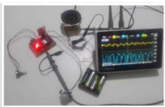
Fig. 11: Measurement of the amplifier circuit with the oscilloscope
