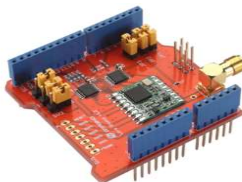
Fig. 2: Dragino Lora Module, [35]
