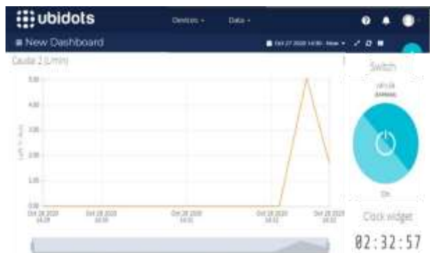
Fig. 13: Valve in ON state in Ubidots (With water flow)
