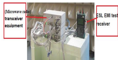
Fig. 4: Measurements on radio frequency common mode immunity
