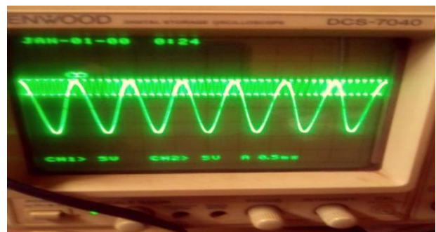
Fig. 16: Experimented waveforms of modulating voltage and positive carrier wave form
