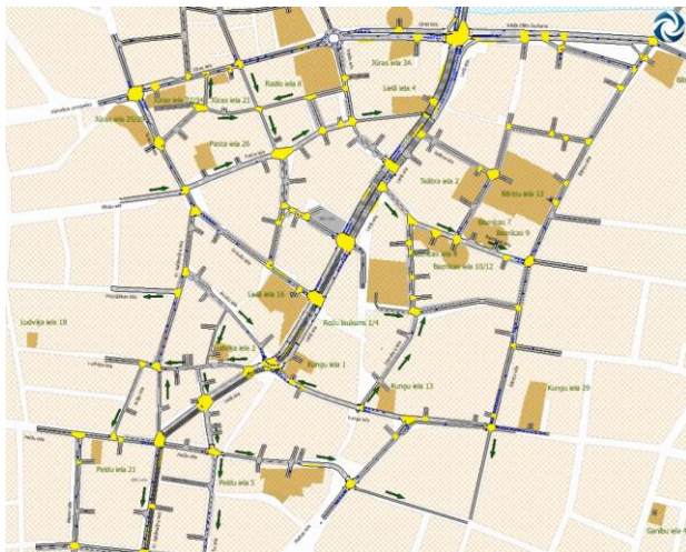
Fig.9. The example of the microscopic transportation simulation model animation in Aimsun tool [38].
