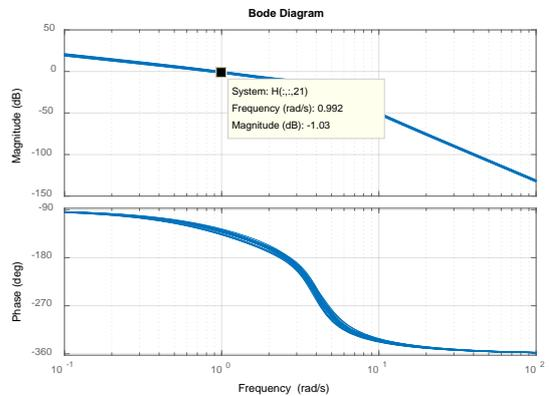
Fig. 4 Bode diagram for open-loop system
