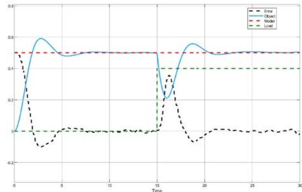
Fig. 6 Transient response graph with exact parameters of controller
