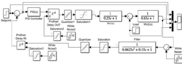
Fig. 2 Mathematical model of a distributed control system.
