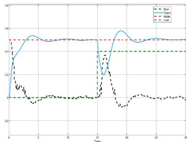
Fig. 7. Transient response graph with 10% variations of controller parameters
