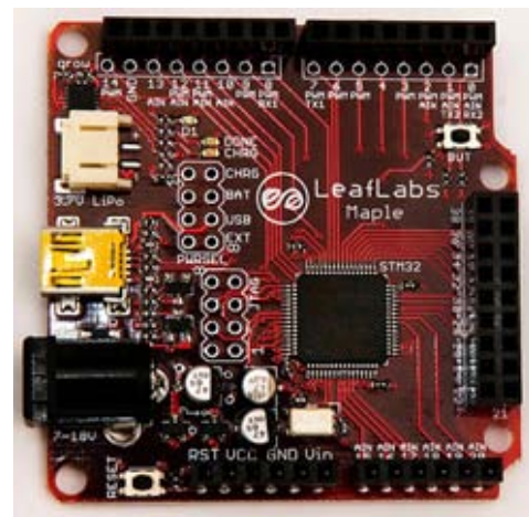
Fig.11 Maple microcontroller board.
