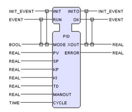
Fig. 7. The PID composite function block
