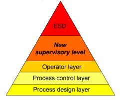
Fig. 1. Layers of protection
