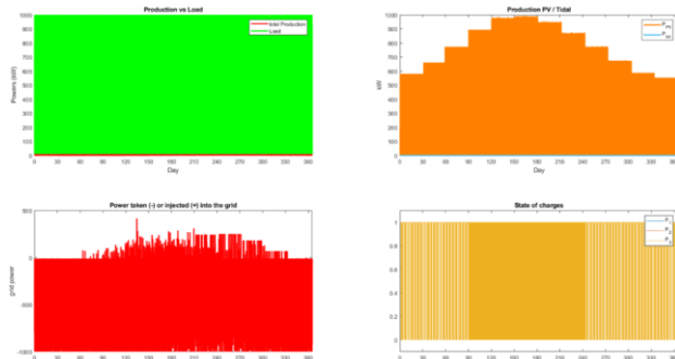
Fig. 15: Evolution of daily production vs load, production PV/Tidal, Power of grid, and state of load (3 rd scenario)
