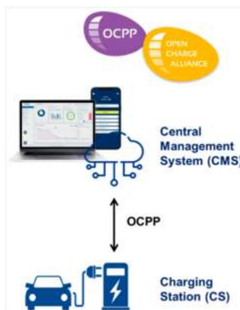
Fig. 1: OCPP is a main communication protocol for data exchange between CMS and CS, [9]
