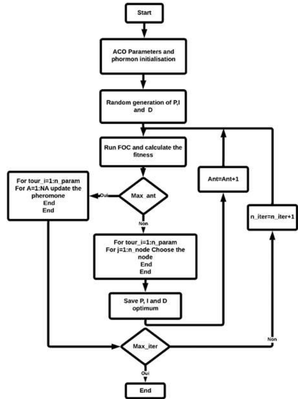
Fig. 5: ACO Sequence for PID Controller optimization
