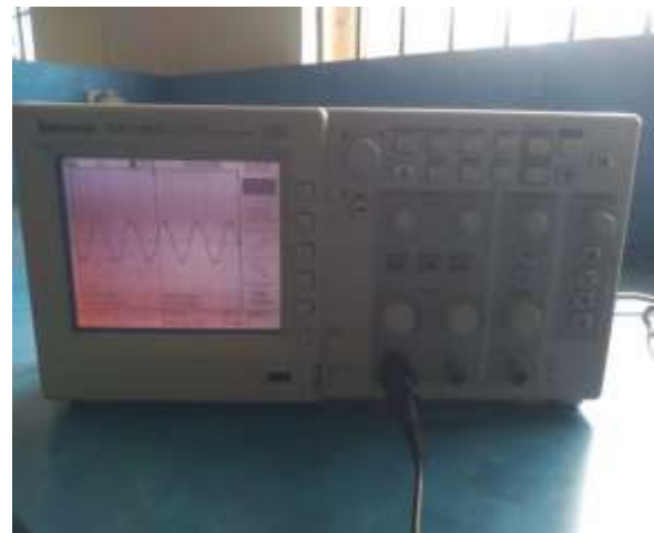
Fig. 18: Grid Output Voltage measured by DSO
