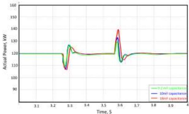
Fig. 5: Reaction of Proposed Model under DC link capacitance different values
