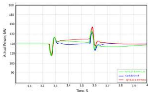
Fig. 6: Reaction of Proposed Model under PI controller parameters different values
