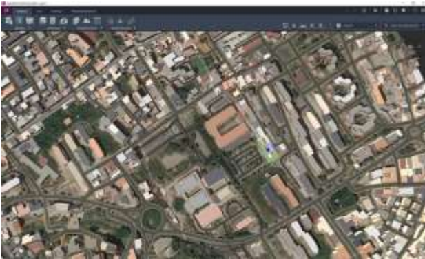
Fig. 9b: Autodesk InfraWorks: visualization of the building correctly georeferenced on the map and of the layers chosen during the modeling phase of the GIS environment in InfraWorks.
