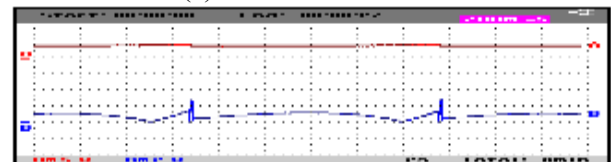
(b) RT-results: Ch. A (Speed) Ch. B (Torque) Fig. 14a,b: Matlab and RT-Lab results for rotor speed and electric torque with STATCOM and three-phase RL impedance.
