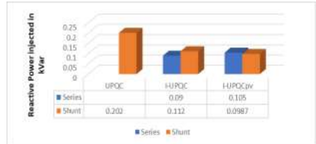
Fig. 19: Imaginary power amelioration for parallel/series inverters in 33-test system
