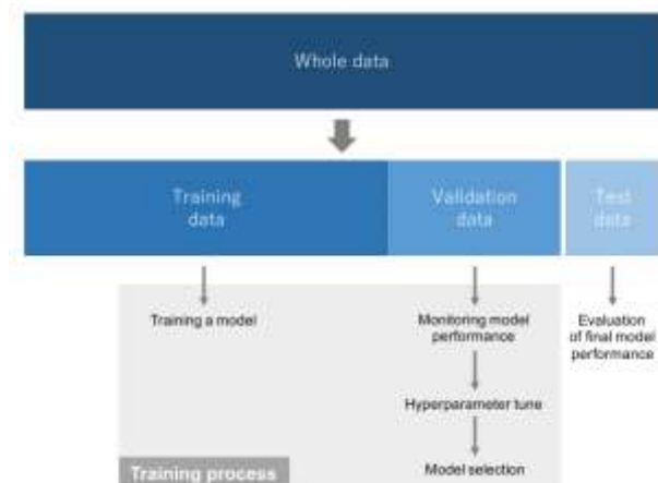
Fig. 2: Available data are typically split into three sets: training, validation, and a test set
