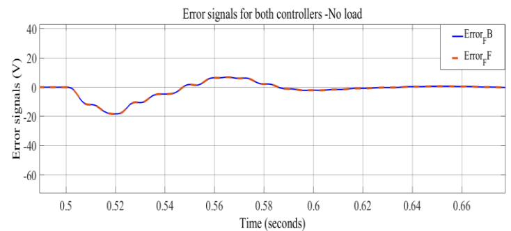
Fig. 7: Error signals of both controllers at 15% disturbance - No load condition.
