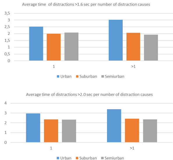
Fig. 6: Average distraction time per number of elements in Urban, Suburban and Semi-urban road environment
