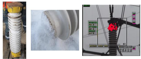
Figure 1. Types of damages to porcelain insulators
