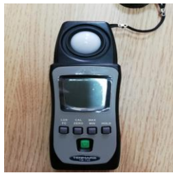
Figure 5. The lux meter used in the experiment
