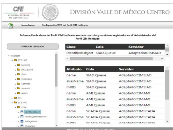
Fig. 9. The Web GUI for Data Model Manager includes a description of ESB queues for each data source integrated by CIM Wrappers.
