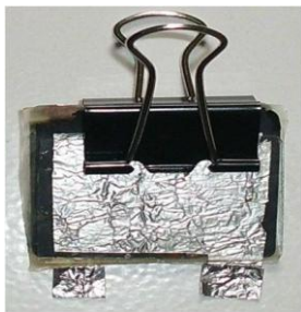
Fig. 4 A simple lithium polymer battery using chitosan membrane as electrolyte matrix
