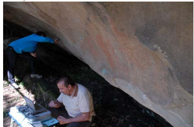
Fig. 2: ASD-FR Spectroradiometer working in field.
