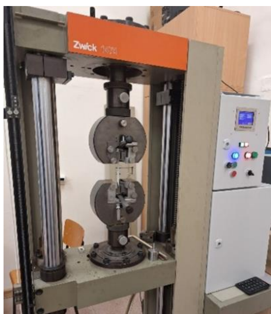
Fig. 5: Tensile testing machine.
