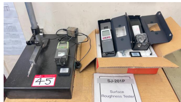
Fig. 4: Surface roughness measurement using a Mitutoyo SJ-201 contact profilometer
