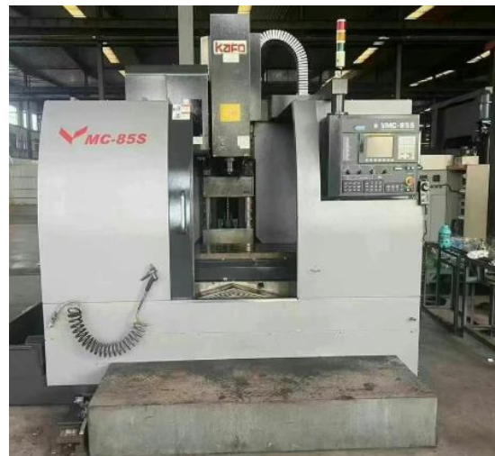
Fig. 3: CNC vertical machining center VMC-85S used for the milling experiments
