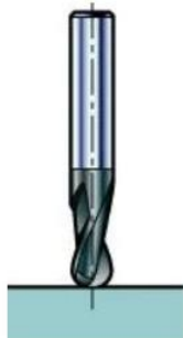
Fig. 2: Geometry of the TiAlN-coated ball-end milling tool used in the experiments
