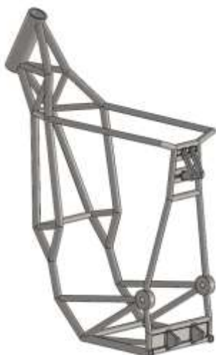
Fig. 10: Tubular frame geometry based on topology optimization result
