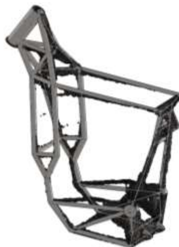
Fig. 11: Comparison of the structure design with the result of topology optimization
