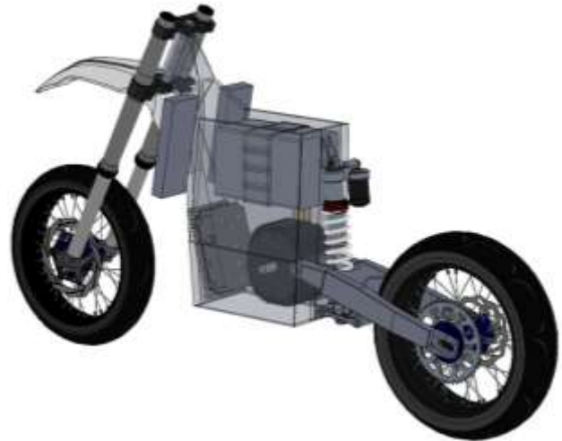
Fig. 1: CAD model of the motorcycle with the assumed geometry of the supporting structure
