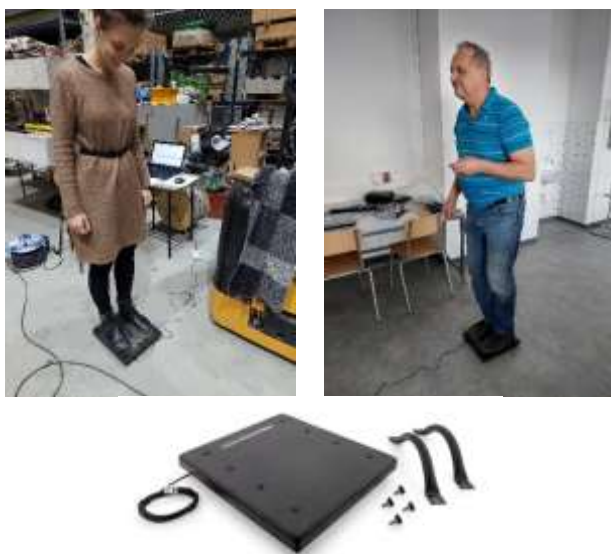
Fig. 10: Two examples of the GRF measurement (top left and top right) and a utilized force plate (bottom middle)
