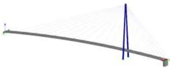
Fig. 6: The 3D computational model of the investigated footbridge in Lužec nad Vltavou
