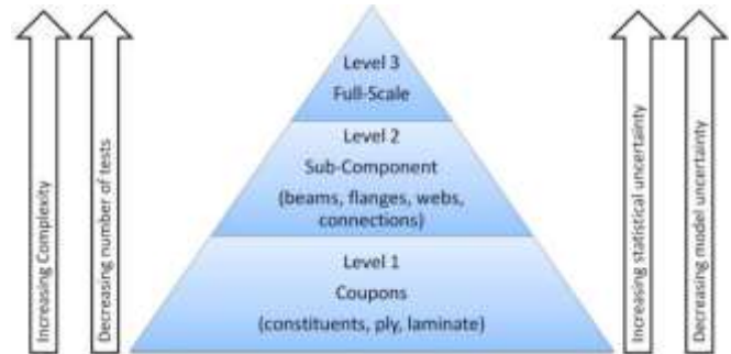
Fig. 1: Levels of wind turbine blade inspections
